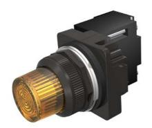
30mm BlackMax, Epoxy Coated Corrosion Resistant Complete Metal Unit Illuminated Indicator Light Transformer type, 480V AC Super Bright LED Lamp, BA9s Glass Lens, Amber UL Listed, CSA Certified NEMA 1,3,3R,4,4X,12,13 & Automotive Standards
