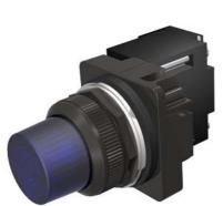
30mm BlackMax, Epoxy Coated Corrosion Resistant Complete Metal Unit Illuminated Indicator Light Transformer type, 480V AC LED Lamp, BA9s Glass Lens, Blue UL Listed, CSA Certified NEMA 1,3,3R,4,4X,12,13 & Automotive Standards
