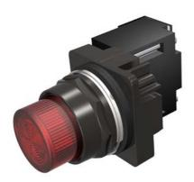
30mm BlackMax, Epoxy Coated Corrosion Resistant Complete Metal Unit Illuminated Indicator Light Full Voltage type, 12V AC/DC Incandescent Lamp, BA9s Plastic Lens, Red UL Listed, CSA Certified NEMA 1,3,3R,4,4X,12,13 & Automotive Standards
