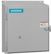
Reversing NEMA contactor, Size 3, Three phase full voltage, Contactor amp rating 90A, 3 wire (NO aux included), 190-220/220-240V 50/60Hz coil, Non-combination type, Encl. NEMA type 4X fiberglass, Water/dust tight noncorrosive, Standard width enclosure
