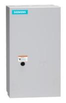
Reversing NEMA contactor Size 3 Three phase full voltage Contactor amp rating 90Amp 3 w 380-440/440-480V 50/60HZ coil Non-combination type Enclosure NEMA type 1 Indoor general purpose use Standard width enclosure
