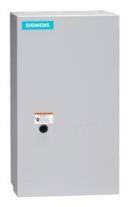
Reversing NEMA contactor Size 3 Three phase full voltage Contactor amp rating 90Amp 3 w 208VAC 60HZ coil Non-combination type Enclosure NEMA type 1 Indoor general purpose use Standard width enclosure
