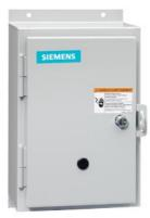
Reversing NEMA contactor Size 1 Three phase full voltage Contactor amp rating 27Amp 3 w 240V 50HZ / 277V 60HZ coil Non-combination type Enclosure NEMA type 12 Dust/drip proof for indoors Standard width enclosure
