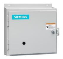
Reversing NEMA contactor Size 0 Three phase full voltage Contactor amp rating 18Amp 3 w 240V 50HZ / 277V 60HZ coil Non-combination type Enclosure NEMA type 12 Dust/drip proof for indoors Standard width enclosure
