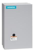
Reversing NEMA contactor Size 00 Single phase full voltage Contactor amp rating 9Amp 3 wi 110V 50HZ / 120V 60HZ coil Non-combination type Enclosure NEMA type 1 Indoor general purpose use Standard width enclosure
