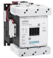
Vacuum NEMA contactor, Size 5, Three phase full voltage, Contactor amp rating 270A, 3 wire (NO aux included), 440-480V 50-60Hz/DC coil, Non-combination type, Enclosure NEMA type (open), No enclosure
