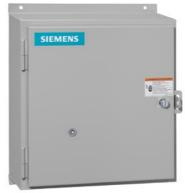
Non-reversing NEMA contactor, Size 3, Three phase full voltage, Contactor amp rating 90A, 3 wire (NO aux included), 190-220/220-240V 50/60Hz coil, Noncombination type, Encl. NEMA type 4X fiberglass, Water/dust tight noncorrosive, Standard width enclosure
