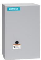
Non-reversing contactor, Size 2 1/2, Three phase full voltage, Contactor amp rating 60A, 3 wire (NO aux included), 190-220/220-240V 50/60Hz coil, Non-combination type, Enclosure NEMA type 1, Indoor general purpose use, Extra-wide enclosure
