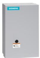
Non-reversing contactor, Size 2 1/2, Three phase full voltage, Contactor amp rating 60A, 3 wire (NO aux included), 110V 50Hz / 120V 60Hz coil, Non-combination type, Enclosure NEMA type 1, Indoor general purpose use, Extra-wide enclosure
