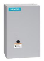
Non-reversing contactor, Size 2 1/2, Three phase full voltage, Contactor amp rating 60A, 3 wire (NO aux included), 208VAC 60Hz coil, Non-combination type, Enclosure NEMA type 1, Indoor general purpose use, Extra-wide enclosure
