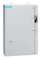
2-speed 3-phase motor starter Size 1 Two separate windings Constant or variable torque Solid-state overload relays Low SPD OLR range 3-12A High SPD OLR range 5.5-22A 110V 50HZ / 120V 60HZ coil Combination type 25Amp circuit breaker Encl NEMA type 4X 304 S-steel Water/dust tight noncorrosive
