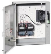
2-speed 3-phase motor starter Size 1 Two separate windings Constant or variable torque Solid-state overload relays Low SPD OLR range 3-12A High SPD OLR range 5.5-22A 110V 50HZ / 120V 60HZ coil Combination type 25Amp circuit breaker Enclosure NEMA type 4/12 Water/dust tight for outdoors
