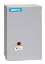
2-speed 3-phase motor starter, Size 1, One winding consequent pole, Constant or variable torque, Solid-state overload relays, Low Spd OLR range 3-12A, High Spd OLR range 5.5-22A, 110V 50Hz / 120V 60Hz coil, Enclosure NEMA type 1, Indoor general purpose use
