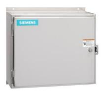
2-speed 3-phase motor starter, Size 1, One winding consequent pole, Constant or variable torque, Solid-state overload relays, Low Spd OLR range 3-12A, High Spd OLR range 5.5-22A, 110V 50Hz / 120V 60Hz coil, Enclosure NEMA type 12, Dust/drip proof for indoors
