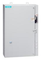
Non-reversing motor starter, Size 1, Three phase full voltage, Solid-state overload relay, OLR amp range 5.5-22A, 24VDC coil, Combination type, 25A circuit breaker, Encl NEMA type 4X 304 S-Steel, Water/dust tight noncorrosive, Extra-wide enclosure
