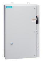
Non-reversing motor starter Size 2 1/2 Three phase full voltage Solid-state overload relay OLRelay amp range 25-100A 240VAC 50HZ / 277VAC 60HZ coil Combination type 100A fusible disconnect 100A/600V fuse clip Encl NEMA type 4X 316 S-steel Water/dust tight non-corrosive Standard width enclosure
