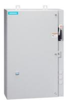
Non-reversing motor starter Size 2 1/2 Three phase full voltage Solid-state overload relay OLRelay amp range 25-100A Combination type 60Amp fusible disconnect 60Amp / 600V fuse clip Encl NEMA type 4X 316 S-steel Water/dust tight non-corrosive Standard width enclosure
