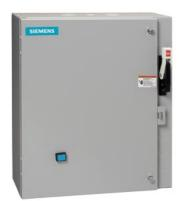
Non-reversing motor starter Size 2 1/2 Three phase full voltage Solid-state overload relay OLRelay amp range 25-100A 380-440/440-480V 50/60HZ coil Combination type 100A fusible disconnect 100A/250V fuse clip Enclosure NEMA type 1 Indoor general purpose use Standard width enclosure
