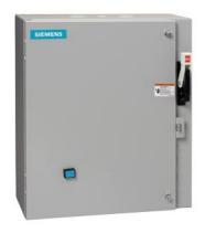
Non-reversing motor starter, Size 2 1/2, Three phase full voltage, Solid-state overload relay, OLR amp range 25-100A, Combination type, 100A fusible disconnect, 100A/600V fuse clip, Enclosure NEMA type 1, Indoor general purpose use, Standard width enclosure
