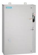
Non-reversing motor starter Size 2 1/2 Three phase full voltage Solid-state overload relay OLRelay amp range 25-100A Combination type 60Amp fusible disconnect 60Amp / 600V fuse clip Encl NEMA type 4X 316 S-steel Water/dust tight non-corrosive Extra-wide enclosure
