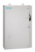
Non-reversing motor starter, Size 2 1/2, Three phase full voltage, Solid-state overload relay, OLR amp range 25-100A, Combination type, 100A fusible disconnect, 100A/600V fuse clip, Encl NEMA type 4X 304 S-Steel, Water/dust tight noncorrosive, Extra-wide enclosure
