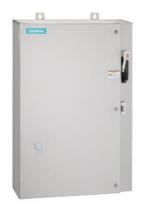
Non-reversing motor starter Size 2 Three phase full voltage Solid-state overload relay OLRelay amp range 13-52a 24Vdc coil Combination type 60Amp fusible disconnect 60Amp / 600V fuse clip Encl NEMA type 4X 316 S-steel Water/dust tight non-corrosive Extra-wide enclosure
