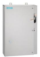
Non-reversing motor starter Size 2 Three phase full voltage Solid-state overload relay OLRelay amp range 13-52a Combination type 60Amp non-fused disconnect Encl NEMA type 4X 316 S-steel Water/dust tight non-corrosive Extra-wide enclosure
