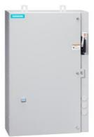
Non-reversing motor starter, Size 2, Three phase full voltage, Solid-state overload relay, OLR amp range 13-52A, Combination type, 60A fusible disconnect, 60A/600V fuse clip, Encl NEMA type 4X 304 S-Steel, Water/dust tight noncorrosive, Extra-wide enclosure
