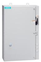
Non-reversing motor starter, Size 2, Three phase full voltage, Solid-state overload relay, OLR amp range 13-52A, Combination type, 60A non-fusible disconnect, Enclosure NEMA type 4/12, Water/dust tight for outdoors, Extra-wide enclosure
