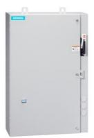
Non-reversing motor starter, Size 2, Three phase full voltage, Solid-state overload relay, OLR amp range 13-52A, 110V 50Hz / 120V 60Hz coil, Combination type, 60A non-fusible disconnect, Enclosure NEMA type 4/12, Water/dust tight for outdoors, Extra-wide enclosure
