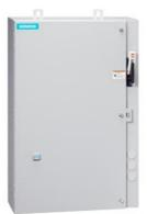
Non-reversing motor starter, Size 2, Three phase full voltage, Solid-state overload relay, OLR amp range 13-52A, 110V 50Hz / 120V 60Hz coil, Combination type, 60A fusible disconnect, 60A/250V fuse clip, Enclosure NEMA type 4/12, Water/dust tight for outdoors, Extra-wide enclosure
