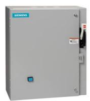
Non-reversing motor starter, Size 2, Three phase full voltage, Solid-state overload relay, OLR amp range 13-52A, 240V 50Hz / 277V 60Hz coil, Combination type, 60A fusible disconnect, 60A/250V fuse clip, Enclosure NEMA type 1, Indoor general purpose use, Extra-wide enclosure
