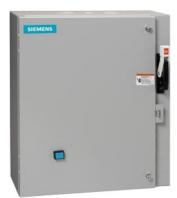
Non-reversing motor starter, Size 2, Three phase full voltage, Solid-state overload relay, OLR amp range 13-52A, Combination type, 60A fusible disconnect, 60A/250V fuse clip, Enclosure NEMA type 1, Indoor general purpose use, Extrawide enclosure
