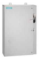
Non-reversing motor starter Size 1 3/4 Three phase full voltage Solid-state overload relay OLRelay amp range 10-40a 240VAC 50HZ / 277VAC 60HZ coil Combination type 60Amp fusible disconnect 60Amp / 600V fuse clip Encl NEMA type 4X 316 S-steel Water/dust tight non-corrosive Extra-wide enclosure
