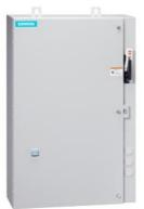
Non-reversing motor starter, Size 1 3/4, Three phase full voltage, Solid-state overload relay, OLR amp range 10-40A, Combination type, 60A fusible disconnect, 60A/600V fuse clip, Encl NEMA type 4X 304 S-Steel, Water/dust tight noncorrosive, Extra-wide enclosure
