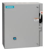
Non-reversing motor starter, Size 1 3/4, Three phase full voltage, Solid-state overload relay, OLR amp range 10-40A, 24VDC coil, Combination type, 60A fusible disconnect, 60A/600V fuse clip, Enclosure NEMA type 1, Indoor general purpose use, Extra-wide enclosure
