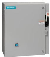
Non-reversing motor starter, Size 1 3/4, Three phase full voltage, Solid-state overload relay, OLR amp range 10-40A, Combination type, 60A fusible disconnect, 60A/250V fuse clip, Enclosure NEMA type 1, Indoor general purpose use, Extrawide enclosure
