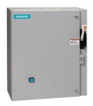
Non-reversing motor starter, Size 1 3/4, Three phase full voltage, Solid-state overload relay, OLR amp range 10-40A, 110V 50Hz / 120V 60Hz coil, Combination type, 60A fusible disconnect, 60A/600V fuse clip, Enclosure NEMA type 1, Indoor general purpose use, Extra-wide enclosure
