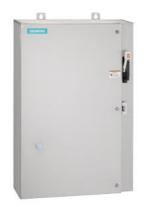
Non-reversing motor starter Size 1 Three phase full voltage Solid-state overload relay OLRelay amp range 10-40a 24Vdc coil Combination type 30Amp fusible disconnect 30Amp / 250V fuse clip Encl NEMA type 4X 316 S-steel Water/dust tight non-corrosive Extra-wide enclosure
