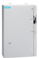
Non-reversing motor starter, Size 1, Three phase full voltage, Solid-state overload relay, OLR amp range 10-40A, 208VAC 60Hz coil, Combination type, 60A fusible disconnect, 60A/250V fuse clip, Encl NEMA type 4X 304 S-Steel, Water/dust tight noncorrosive, Extra-wide enclosure
