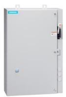
Non-reversing motor starter, Size 1, Three phase full voltage, Solid-state overload relay, OLR amp range 10-40A, Combination type, 60A non-fusible disconnect, Enclosure NEMA type 4/12, Water/dust tight for outdoors, Extra-wide enclosure
