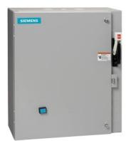
Non-reversing motor starter, Size 1, Three phase full voltage, Solid-state overload relay, OLR amp range 5.5-22A, Combination type, 30A fusible disconnect, 30A/600V fuse clip, Enclosure NEMA type 1, Indoor general purpose use, Extrawide enclosure
