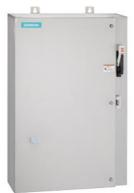
Non-reversing motor starter Size 1 Three phase full voltage Solid-state overload relay OLRelay amp range 3-12A 24Vdc coil Combination type 30Amp fusible disconnect 30Amp / 250V fuse clip Encl NEMA type 4X 316 S-steel Water/dust tight non-corrosive Extra-wide enclosure
