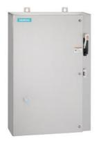
Non-reversing motor starter Size 1 Three phase full voltage Solid-state overload relay OLRelay amp range 3-12A Combination type 30Amp fusible disconnect 30 Amp /600V fuse clip Encl NEMA type 4X 316 S-steel Water/dust tight non-corrosive Extra-wide enclosure
