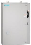
Non-reversing motor starter Size 1 Three phase full voltage Solid-state overload relay OLRelay amp range 3-12A 208VAC 60HZ coil Combination type 30Amp fusible disconnect 30Amp / 250V fuse clip Encl NEMA type 4X 316 S-steel Water/dust tight non-corrosive Extra-wide enclosure
