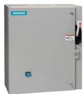
Non-reversing motor starter, Size 1, Three phase full voltage, Solid-state overload relay, OLR amp range 3-12A, Combination type, 30A fusible disconnect, 30A/600V fuse clip, Enclosure NEMA type 1, Indoor general purpose use, Extra-wide enclosure
