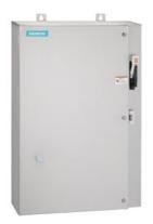
Non-reversing motor starter Size 1 Three phase full voltage Solid-state overload relay OLRelay amp range 0.75-3.4A 208VAC 60HZ coil Combination type 30Amp fusible disconnect 30Amp / 250V fuse clip Encl NEMA type 4X 316 S-steel Water/dust tight non-corrosive Extra-wide enclosure
