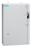
Non-reversing motor starter, Size 1, Three phase full voltage, Solid-state overload relay, OLR amp range 0.75-3.4A, Combination type, 30A fusible disconnect, 30A/600V fuse clip, Encl NEMA type 4X 304 S-Steel, Water/dust tight noncorrosive, Extra-wide enclosure
