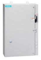
Non-reversing motor starter, Size 1, Three phase full voltage, Solid-state overload relay, OLR amp range 0.75-3.4A, Combination type, 30A fusible disconnect, 30A/250V fuse clip, Enclosure NEMA type 4/12, Water/dust tight for outdoors, Extra-wide enclosure
