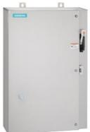
Non-reversing motor starter Size 1 Three phase full voltage Solid-state overload relay OLRelay amp range 0.25-1A 24Vdc coil Combination type 30Amp fusible disconnect 30Amp / 250V fuse clip Encl NEMA type 4X 316 S-steel Water/dust tight non-corrosive Extra-wide enclosure
